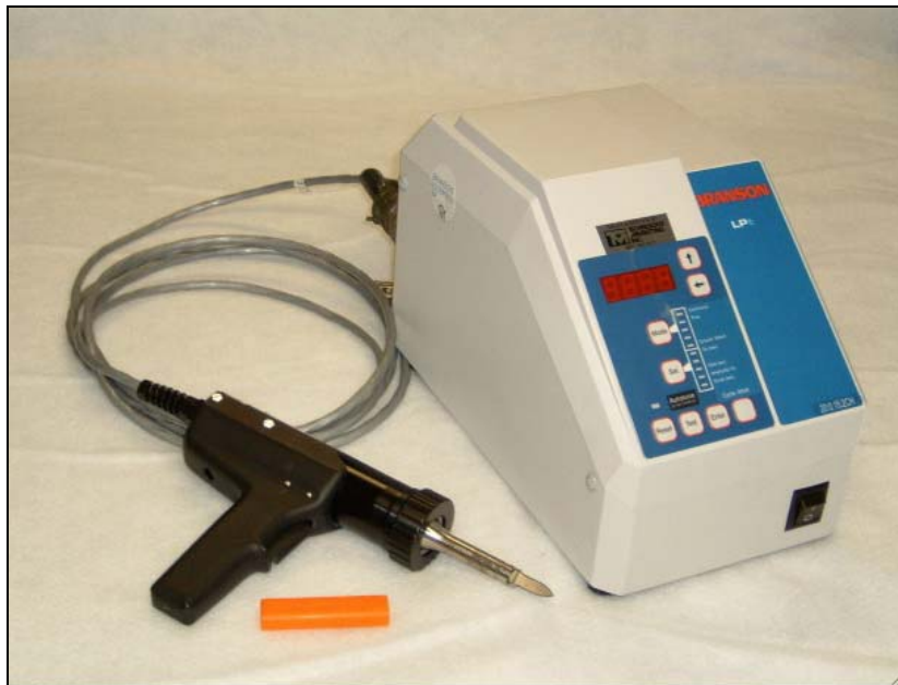
ULTRASONIC TRIM KNIFE (UTK) - 2000LPt (Power Supply: 9" high, 7.75" wide, 13.3" deep)
