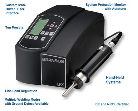
Using the Branson LPX, 150 watt variable amplitude power supply, offers control of the amplitude (blade stroke) for different materials and thicknesses. The system is capable of both constant and timed ultrasonic activation. A choice of steel, carbide, or titanium tips and blades provide the accessories necessary to complete a variety of composite cutting operations.
